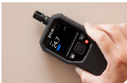
Verify moisture with Pinless measurements
